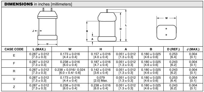
Note: The anode termination (D less B) will be a minimum of 0.012" [0.3 mm]
